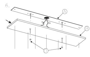
Remove rods  $\bigcirc$  and attach  $\bigcirc$  to  $\bigcirc$  with the button head screws  $\bigcirc$
